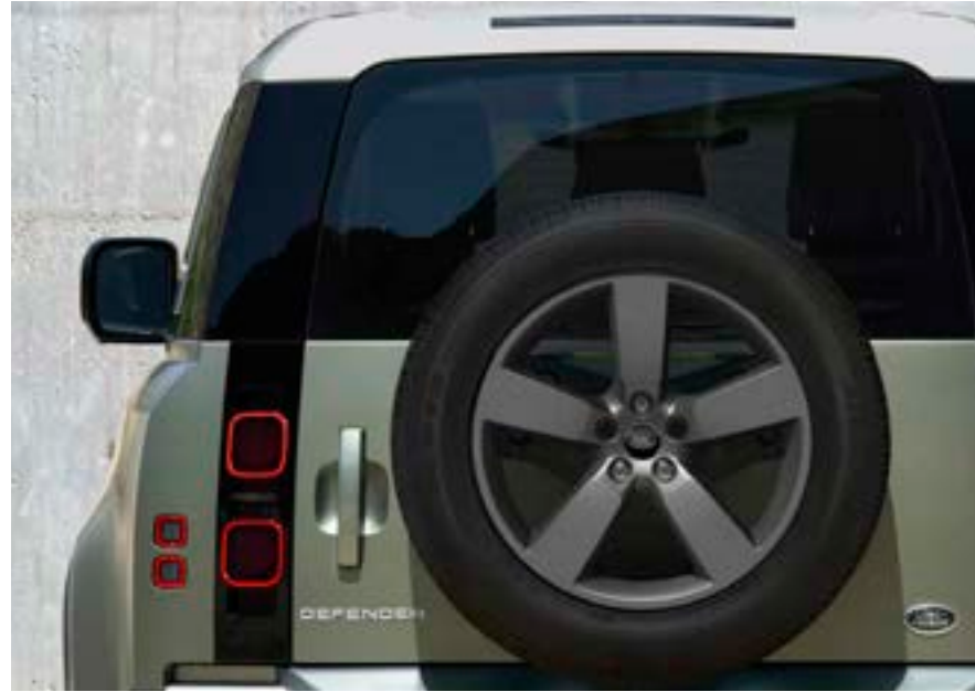
20" STYLE 5098, 5 SPOKE, SATIN DARK GREY Off-road tyres are required if fitted on V8 models.
